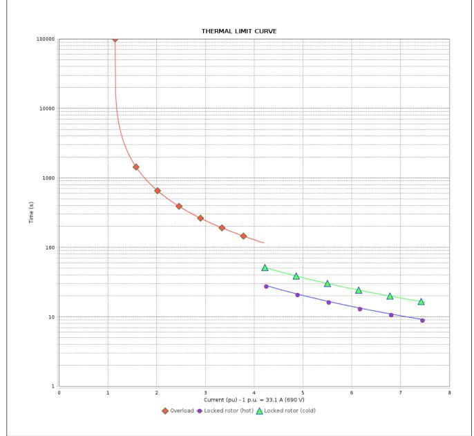
Performance : 400/690 V 50 Hz 4P : 57.1/33.1 A Moment of inertia (J) : 0.3202 kgm<sup>2</sup> Rated current **LRC** : 7.5 Duty cycle : S1 Insulation class : 194 Nm : F Rated torque : 280 % Locked rotor torque Service factor : 1.00 Breakdown torque : 310 % : 80 K Temperature rise Rated speed : 1480 rpm Design : N Heating constant Cooling constant
