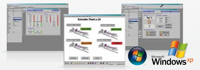
Extremely easy and intuitive, Vedowin is the configuration environment for SCADA/HMI solutions for supervision and management of data from different systems or factory departments. In addition to connection to work stations with Gefran architecture, there are a series of drivers (communication protocols) for the principal devices and instruments used in industrial automation networks.
