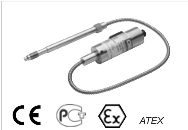
The MX series of Gefran, are pressure transmitters for using in High temperature environment. The main characteristic of this series is the capability to read temperature of the media up to 400°C. The constructive principle is based on the hydraulic transmission of the pressure. The fluid-filled system assures the temperature stability. The physical measure is transformed in a electrical measure by means the strain-gauge technology.
