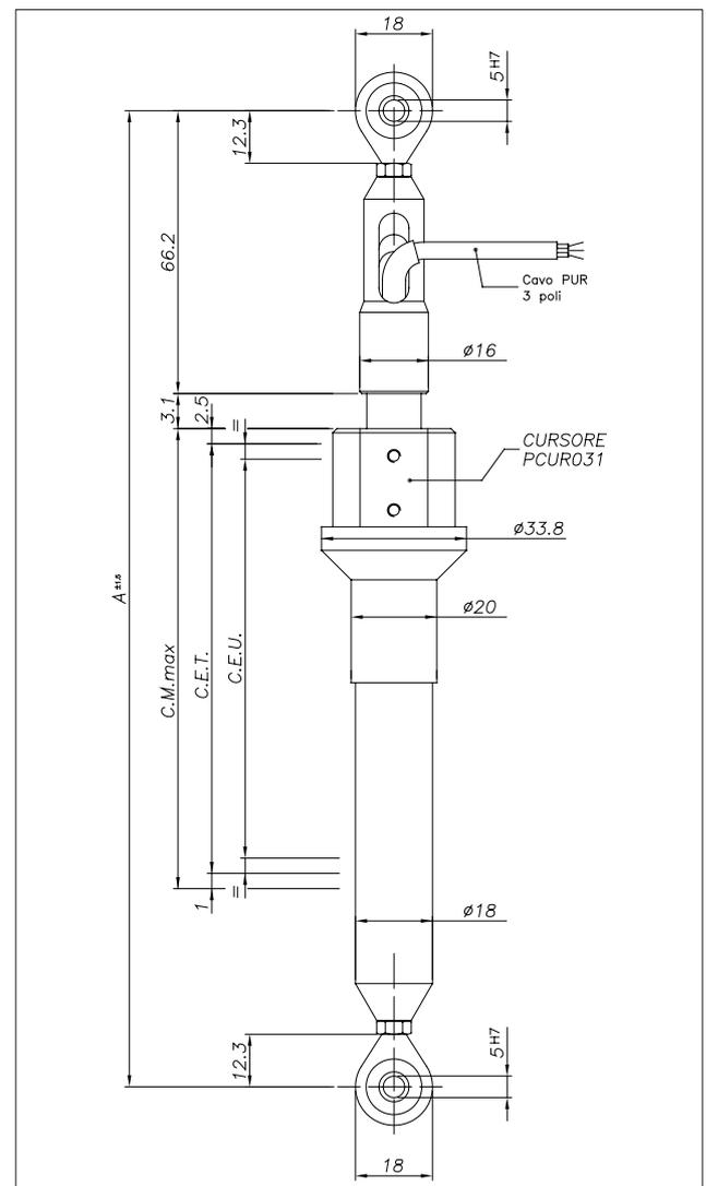
**Important:** all data shown in the catalog for linearity values and temperature coefficients are valid when the sensor is used as voltage divider with maximum current of  $I_c < 0.1 \mu A$  in the circuit.
