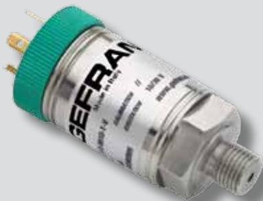
Thanks to a silicon piezoresistive sensitive part, the TSA series is able to measure very low ranges, from 0-50 mbar (0-50 cmH<sub>2</sub>O) or 0-100 mbar (0-1 mH<sub>2</sub>O).
