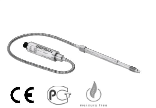
The W3 series of Gefran, are pressure transducers for using in High temperature environment. The main characteristic of this series is the capability to read temperature of the media up to 315°C. The constructive principle is based on the hydraulic transmission of the pressure. The fluid-filled system assures the temperature stability. The physical measure is transformed in a electrical measure by means the strain-gauge technology.
