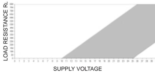
The diagram shows the optimum ratio between the load and supply voltage of the 4...20mA transmitter. For a correct use, choose any combination of load resistance and supply voltage, in the shaded area.
