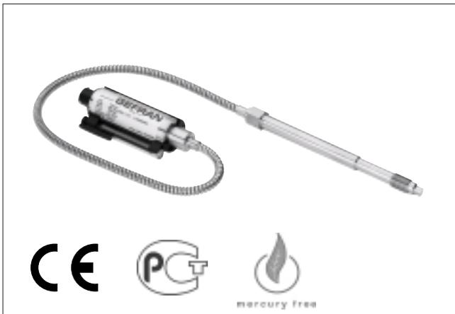
The WE series of Gefran, are pressure transmitters for using in High temperature environment. The main characteristic of this series is the capability to read temperature of the media up to 315°C. The constructive principle is based on the hydraulic transmission of the pressure. The fluid-filled system assures the temperature stability. The physical measure is transformed in a electrical measure by means the strain-gauge technology.
